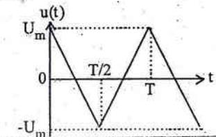
$$U_{\text{eff}} = \sqrt{\frac{1}{T} \int_0^T u^2(t) dt} = \sqrt{\frac{1}{T} \left[ \int_0^{T/2} \left( -\frac{4U_m}{T} t + U_m \right)^2 dt + \int_{T/2}^T \left( \frac{4U_m}{T} t - 3U_m \right)^2 dt \right]}$$
