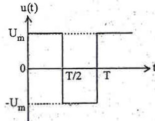
$$U_{\text{eff}} = \sqrt{\frac{1}{T} \int_0^T u^2(t) dt} = \sqrt{\frac{1}{T} \left[ \int_0^{T/2} U_m^2 dt + \int_{T/2}^T (-U_m)^2 dt \right]} = \sqrt{\frac{U_m^2}{T} \left( \frac{T}{2} + \frac{T}{2} \right)}$$
